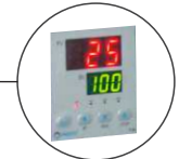
Microprocessor based PID temperature controller
